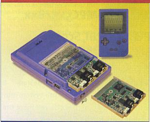
The ready built GBDSO board costs £ 90.00 including the associated PC software and the magazine articles The GBDSO (Gameboy Digital Sampling Oscilloscope), published in Elektor Electronics October and November 2000 is still in great demand.
